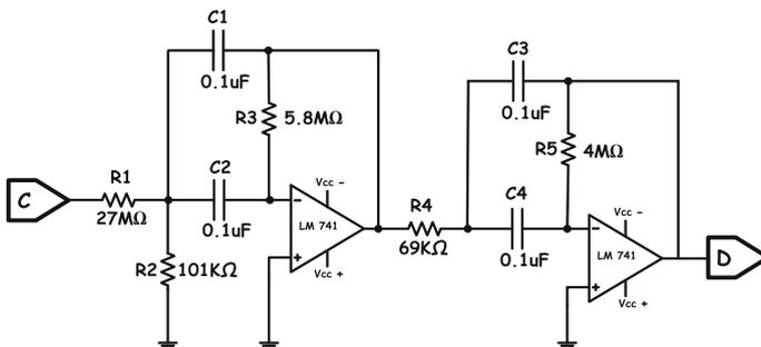
Fig. 47.2 Chebyshev band pass filter
